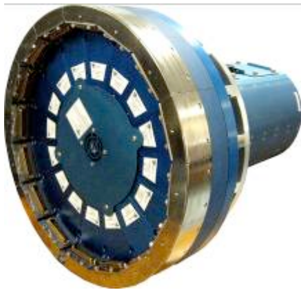
RMDATS assembly (16 DAS segments; 256 dynamic channels)
