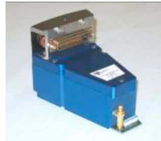
16 channel Data Acquisition Segment (DAS)
